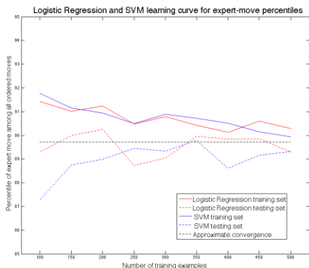
Figure 3: The above learning curves show that the SVM and logistic regression models similarly suffer from high bias. The average percentiles of the expert moves converge to about 90%, only marginally better than the Naive Bayes average of 86%.
